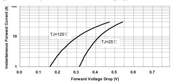
Fig.3-Typical Instantaneous Forward Voltage Characteristics
